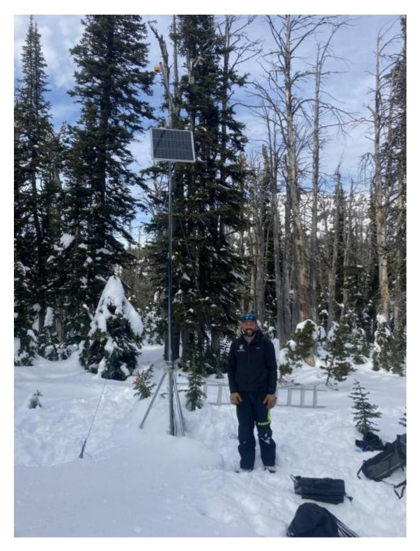
Went to do maintenance on the Sawtelle Snowfall weather station at 8800 ft just off the Sawtelle Mountain Road. Continuous snowcover starts around 8000 ft. At 8800 ft there is  $\sim$ 20" of snow with a mix of hard crusts and weak facets. These weak layers near the ground will be something to watch once snows again. Photo: GNFAC
