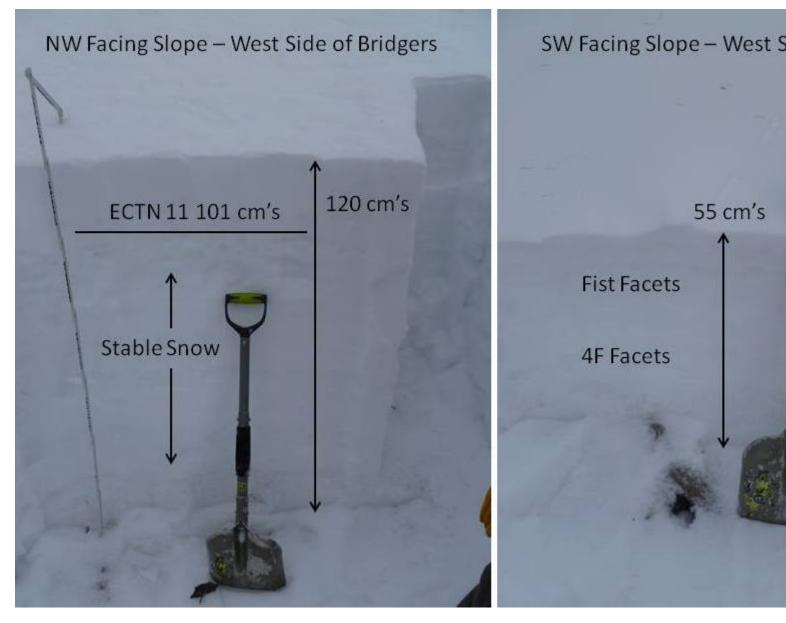
Snow conditions vary widely from slope to slope on the west side of the Bridger Range. These pits were dug only 50 meters apart, but show completely different snowpacks. Photo GNFAC
