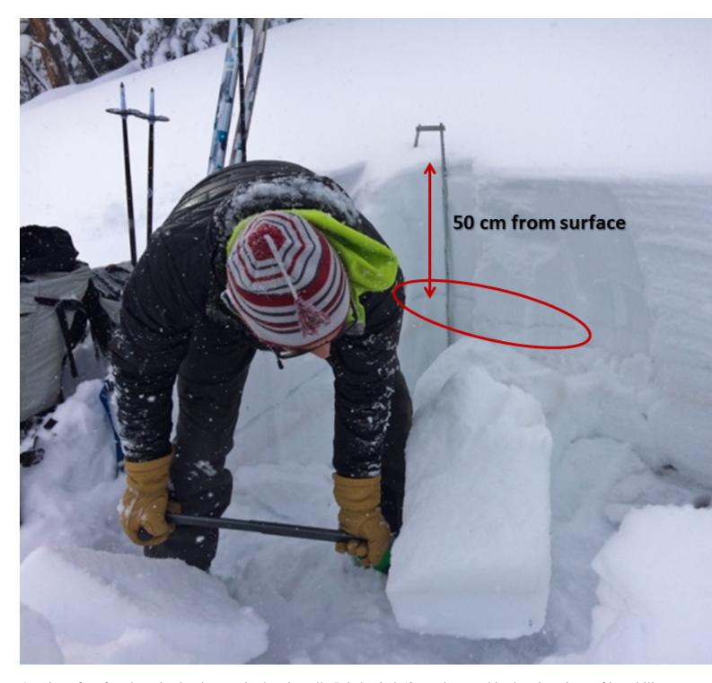
A stripe of surface hoar is clearly seen in the pit wall. It is buried 50 cm deep and is showing signs of instability in our Extended Column Tests (ECTP 12, 14 and 15). Photo: A. Fauver
